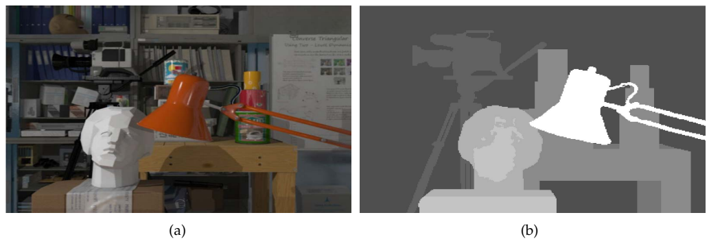
Figure 4. (a) Head and Lamp Image, (b) Depth map of the image. (adapted from the Tsukuba Stereo Vision dataset [37])
